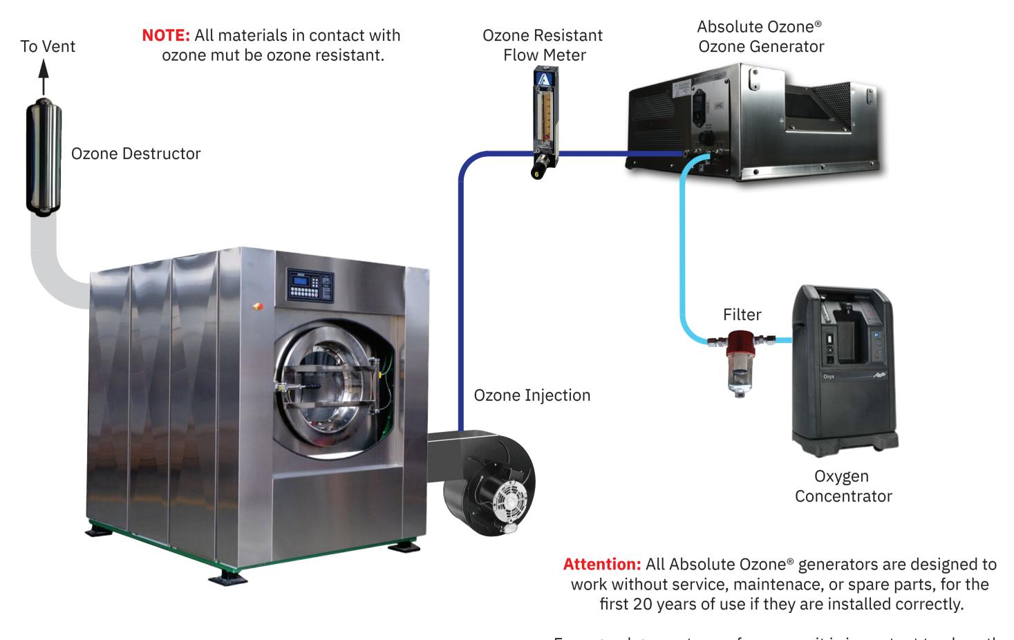
For a good generator performance, it is important to place the generator in a well-ventilated, duat free environment, and mantain the ambient temperature at 20-22 °C
