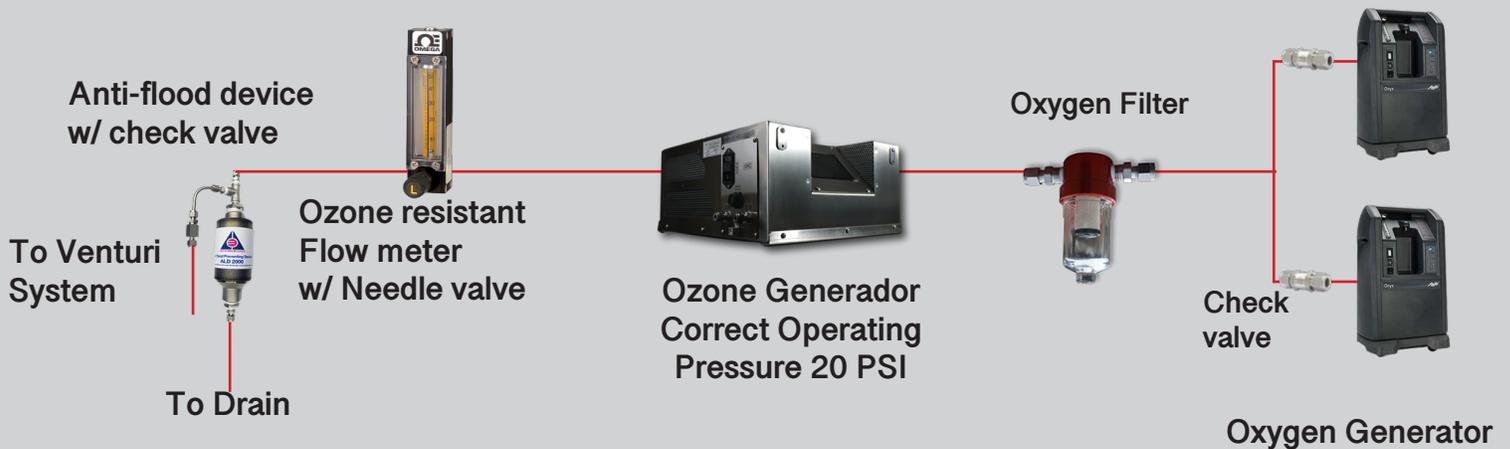
The low-pressure version of the Atlas 60 only required two standard oxygen generators, such as an Onyx Ultra (10 LPM at 20 PSIG each). Eliminating the need for a more sophisticated oxygen generator and air compressor. Atlas 60 low pressure is ideal when high pressure is not a process requirement
