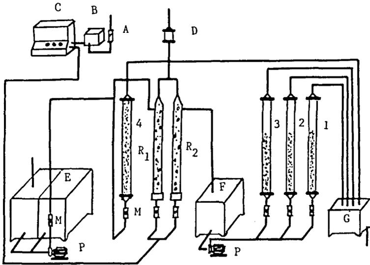
**Legend:** A - dryer-filter; B - oil-free compressor; C - ozone generator; D - GAC reactor; 1 - activated carbon column; 2 - activated carbon/sand column; 3 - sand filtration column; 4 - activated carbon column; E - raw water storage and adjusting tanks; F - intermediate storage tank for ozonated water; G - purified water sampling tank; M - rotameter; P - pumps; R<sub>1</sub> and R<sub>2</sub> - ozonation reactor.
