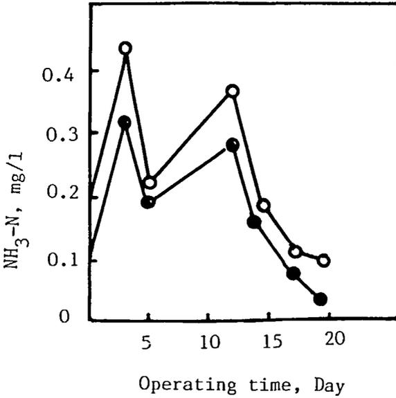
Figure 4. NH<sub>3</sub>-N content curves for raw water (lower) and ozonated water (upper).
