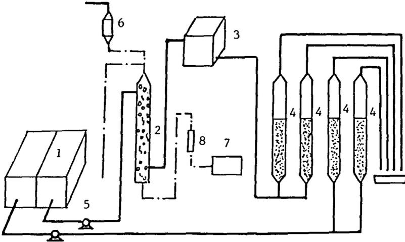
**Legend:** 1 - raw water tank; 2 - ozonation reaction column; 3- intermediate high level water tank; 4 - activated carbon columns; made of glass, 2.4 cm diameter x 1.5 m height; columns I and III packed with activated carbon X-11, 60 cm in depth; columns II and IV packed with activated carbon ZJ-15, 90 cm in depth; 5- pumps; 6 - activated carbon adsorber for residual ozone; 7- ozone generator; 8 - rotameter.
