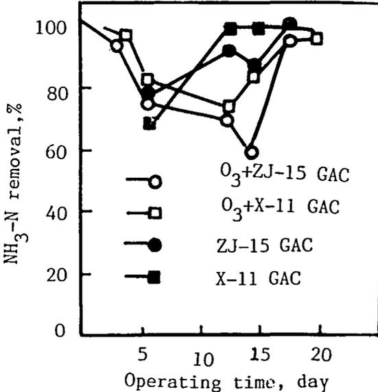
Figure 5. NH<sub>3</sub>-N removal curves for "O<sub>3</sub>-BAC" and "BAC" processes.
